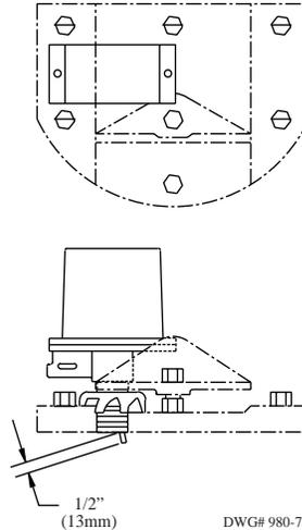
**Typical Pressure Reducer Type Valve Installation**
