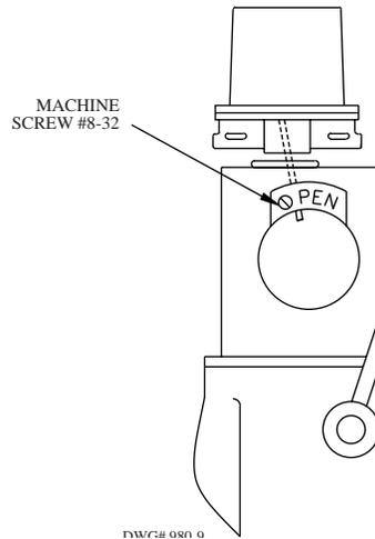
Pratt Valve Kit as used to mount a PCVS on a Pratt Model PIVA Valve.
