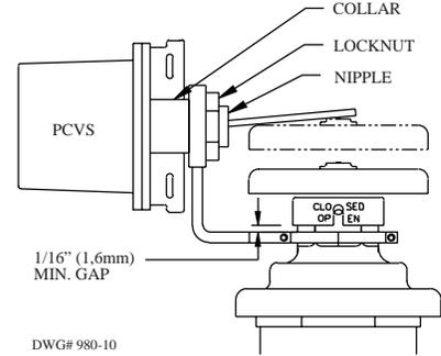
This figure shows the Model PCVS mounted on the valve yoke, with a bracket supplied by the valve manufacturer, to supervise a pressure reducer type valve.
