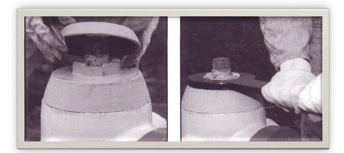
Clow's Body Cap Wrench is for use on McAvity M67 fire hydrants with the threaded on bonnet.
