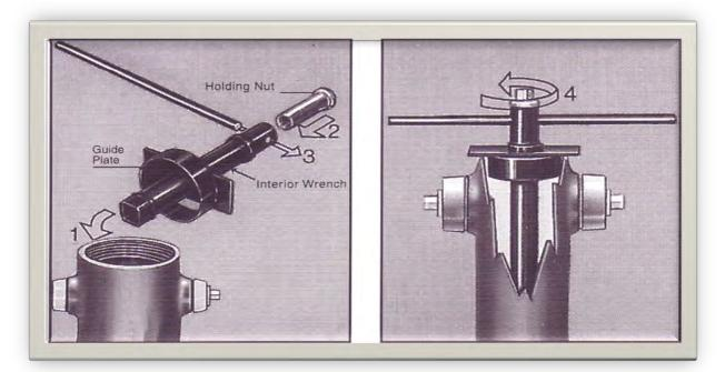
Clow **Seat Removal Tool & Guide Plate** for use on all McAvity hydrants dating back to 1967. (M67 / M67B BRIGADIER / M93B BRIGADIER) check with sales for compatibility with other Clow Canada Hydrants.
