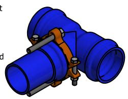
2. Use the restraining rod as a guide and position the 300C split clamp on the pipe. Place hex head clamp bolts through clamp ears insuring bolt end threads are exposed. DO NOT TIGHTEN CLAMP BOLTS, LEAVE LOOSE.
