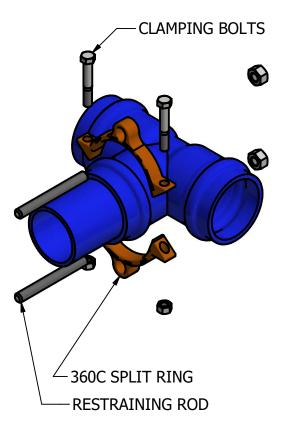
1. Install pipe into the fitting per the pipe manufacturer's instructions. Place the 360C split ring behind the fittings gasket races clamping the halves together. Insert the restraining rods into each 360C split ring placing a nut on each rod behind the ring.
