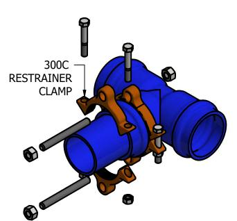
**3.** Align the restraining rods and insure equal threads are beyond the 360C ring and the 300C clamp. Tighten the clamping bolts and nuts insuring equal gaps exist between the two halves. Torque clamping bolts to the following torque requirements:
