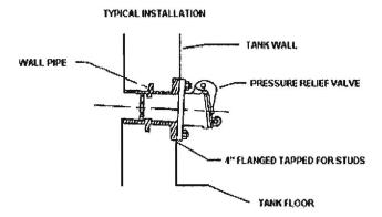
• The valve shall be manufactured using a cast iron body and disc. The seat shall be bronze and the replaceable cover seat shall be BUNA-N. The valve shall be the model A2580 or an approved equal. The diameter of the valve shall be 4" or 6".
